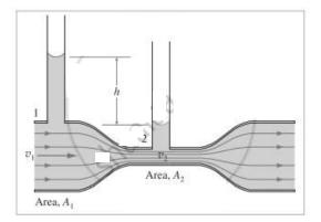
Let A<sub>1</sub> and A<sub>2</sub> be the cross-sectional areas at points 1 and 2, respectively. Let  $v_1$  and  $v_2$  be the corresponding flow speeds.  $\rho$  is the density of the fluid in the pipeline. By the equation of continuity,
