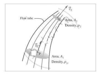
Consider a fluid in steady or streamline flow, that is its density is constant. The velocity of the fluid within a flow tube, while everywhere parallel to the tube, may change its
